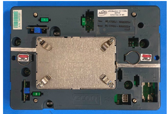
CableServ C-Cor NL Series Band Split to Mid-Split/High-Split Upgrade
