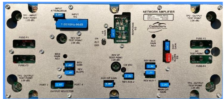
CableServ TNA Mid-Split Upgrade Module
