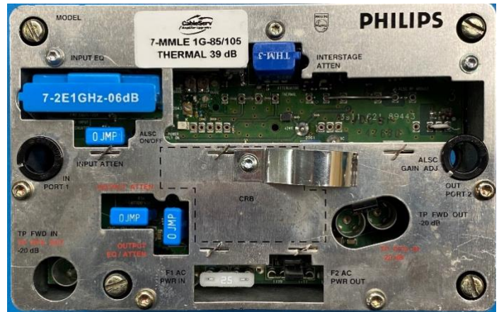
CableServ 7MMLE Series FW and Band-Split Upgrade
