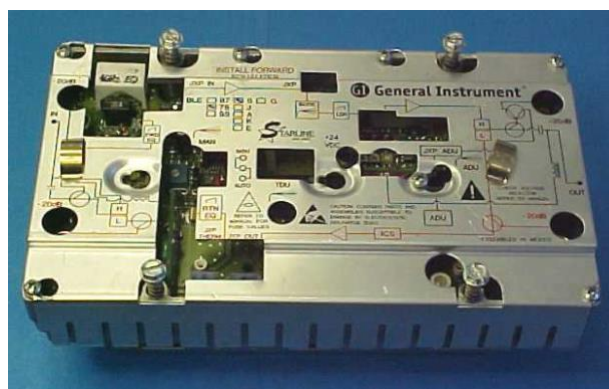
CableServ BLE-S series, 1 GHz Mid/High Split Upgrade
