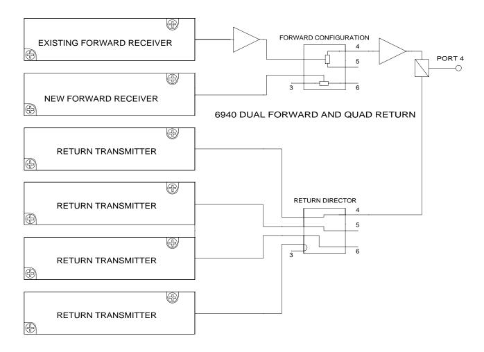
Dual Forward segmentation is as shown above. The new Return Interstage directs each port to an individual laser location. The upper right port is directed to the existing laser location.
