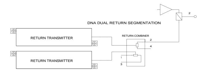
No alteration to the base 6DNA is required. The segmentation can be performed with the amplifier in operation, and only momentary Return Path interruptions.
