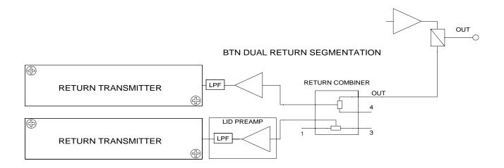
No alteration to the base BT Node is required. The segmentation can be performed with the amplifier in operation, and only momentary Return Path interruptions.
