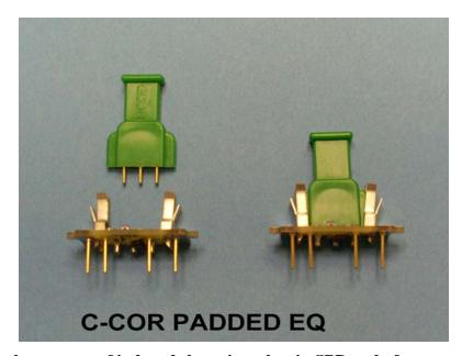
The Resistive element, which determines the amount of induced slope, is a plug-in SPB pad of the same type usually employed for level attenuation in the amplifier model. The technician simply plugs in the common EQ carrier and then the correct value pad.
